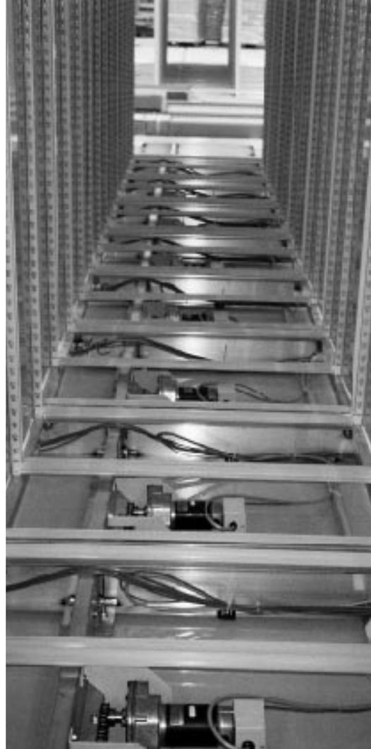
The carriages feature a welded aluminum uniframe construction, which provides a high strength-to-weight ratio; prevents binding, racking, and misalignment; and eliminates the need for fasteners that can loosen or break.
